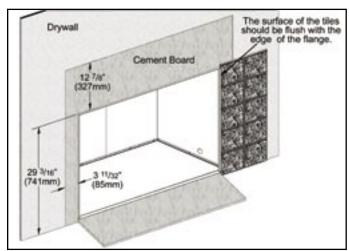
Figure 16. Dimensions Facing Around Opening.
